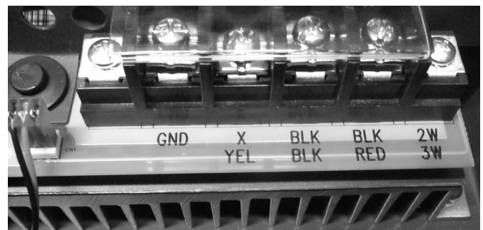
1Ø - 2W/3W Wires to Motor
